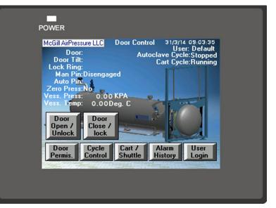
Easy to read, logical control screens give the operator complete control over all autoclave functions.
