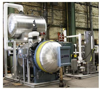
McGill AirPressure's dewaxing autoclave systems are delivered as a complete, ready-to-install package.
