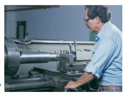
Replacement fan shafts are manufactured to original specifications.
