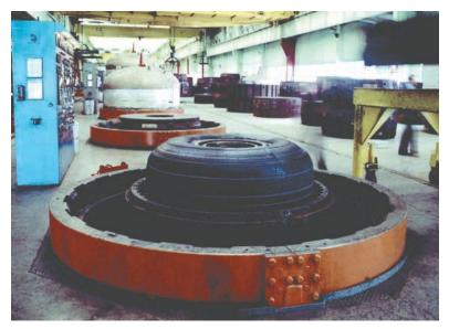
McGill AirPressure designed and manufactured this series of rubber curing autoclaves for a major supplier of large off-the-road tires.
