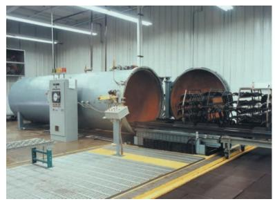
This McGill AirPressure vulcanizing autoclave system, which included the bridge, load carts, and control system, is used to manufacture specialty rubber hose.
