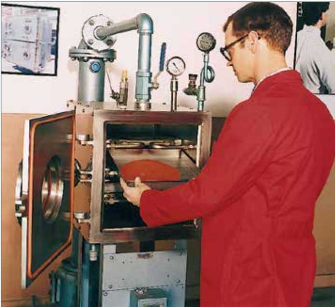
Pilot-sized vacuum dryers can be used to determine what type and size dryer is right for your applications.
