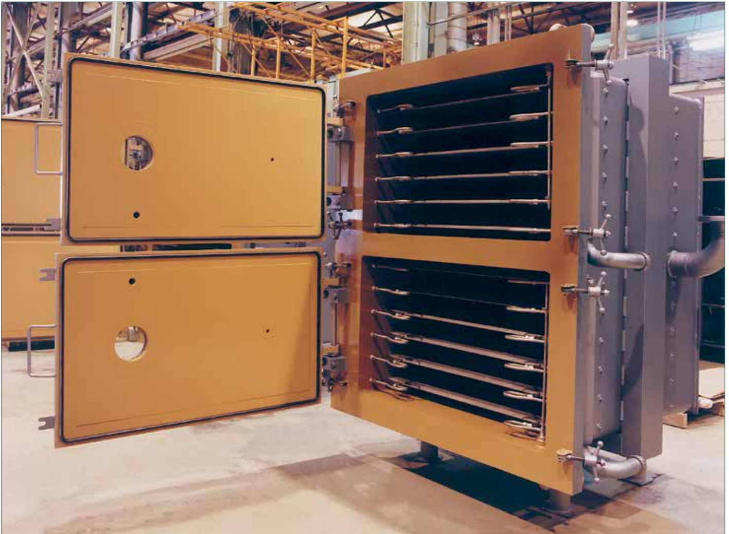
A vacuum shelf dryer designed with two independent chambers for drying two types of materials at the same time.
