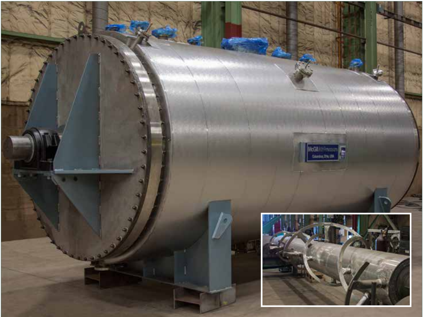
A stainless steel rotary dryer for a chemical processing application. Internal ribbon agitators (inset) help dry materials evenly.
