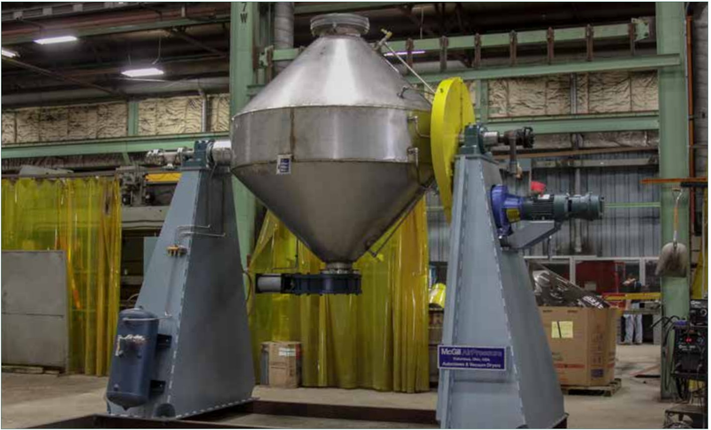
A vacuum conical dryer designed for processing powdered metals.
