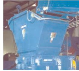
The shredder renders the waste unrecognizable and reduces its volume prior to compaction, optimizing storage capacity of the compactor.
