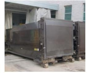
The process is complete when the sterilized shredded waste is compressed by compactors and eventually hauled to a sanitary landfill.
