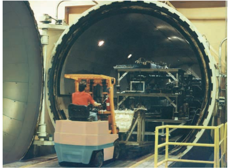
McGill AirPressure installed this 15-foot-diameter by 55-foot-long vessel as part of a twin-autoclave system for a major aircraft manufacturer.
