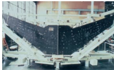
McGill AirPressure's bonding autoclave systems are used to bond a variety of composite materials and products. Pictured (left) is a composite aircraft wing assembly and (right) a composite structural frame for a communication satellite.
